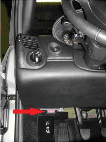
The OBD2 Port is the purple connector on the left side of the steering column below the dash.
